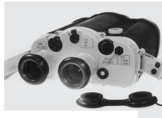
Fotona's top-performance laser range-finder RLD was able to measure distances of up to 30 km by measuring the time of flight of an Nd:YAG laser pulse reflected from a target.
